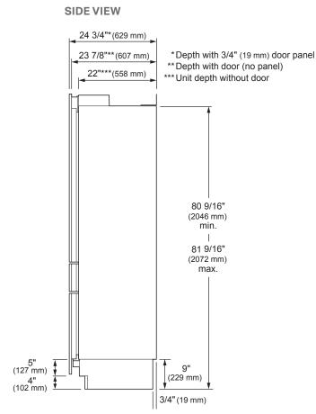
Refer to the Integrated Column Planning/Installation Guide for details on installing multiple columns, door swing dimensions, cabinet planning, retrofit installation and more.
